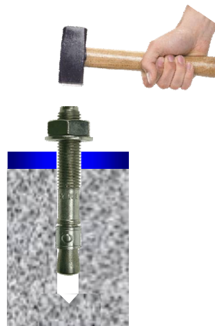
Insert assembled anchor through fixture into concrete
